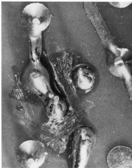
Figure 2. After soldering a new component in place, this person tried to remove the excess solder flux by scraping with a sharp tool. Definitely not acceptable.
