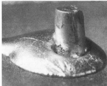
Figure 17. Unacceptable cold solder joint. Lead was moved before solder cooled.
