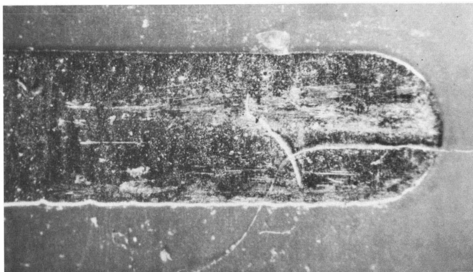
Figure 33. Example of dirty edge connector. Note the crushed fibers and lint from a cotton swab and paper-type cloth.
