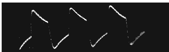
Square Wave Distortion from poor response at both low and high frequency. (A typical amplifier oscillogram.)
