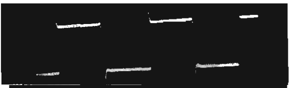
Attenuator leakage at high frequencies shows up in this oscillogram.
