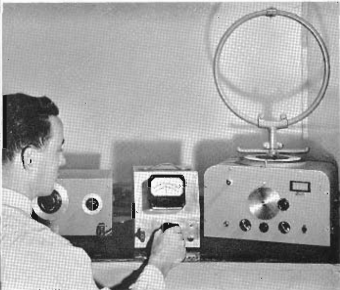
Model 400A is being used for measurements on a Radio Compass.
