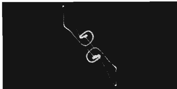
Same as left. One amplifier defective shows up immediately whereas without square wave a long point by point frequency response would be required to discover deviation from standard.
