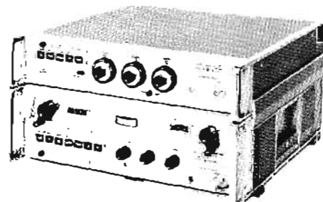
Figure 8. Joining brackets effectively weld instruments into a single physical unit.
