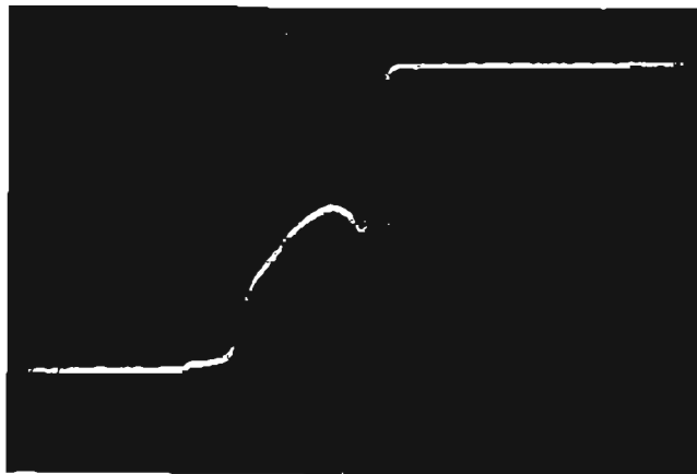
Figure 1. Single-shot transient displayed on Model H30-175A (sweep speed 50 nsec/cm).
