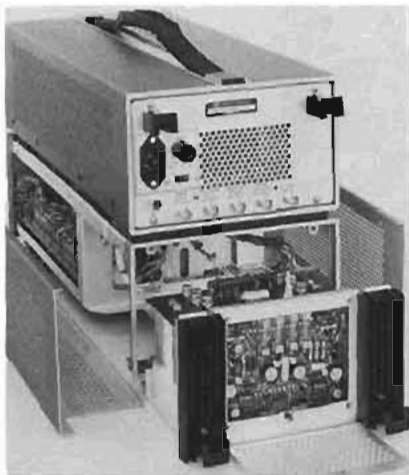
Figure 4. Power supply module can be operated outside the mainframe to facilitate maintenance.
