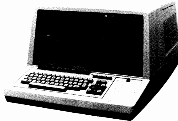
Figure 5. Model 64100A Development Station is the basic unit of the 64000 System. The development station houses all the system options, and is the interface between the user and the Logic Development System. Up to six development stations can be used with a printer and one or more hard discs.
