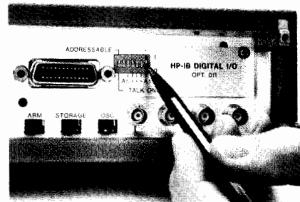
Rear panel switches are set so instrument will either be addressable by controller in a multi-device system, or will simply "talk only" to another device such as a printer.
