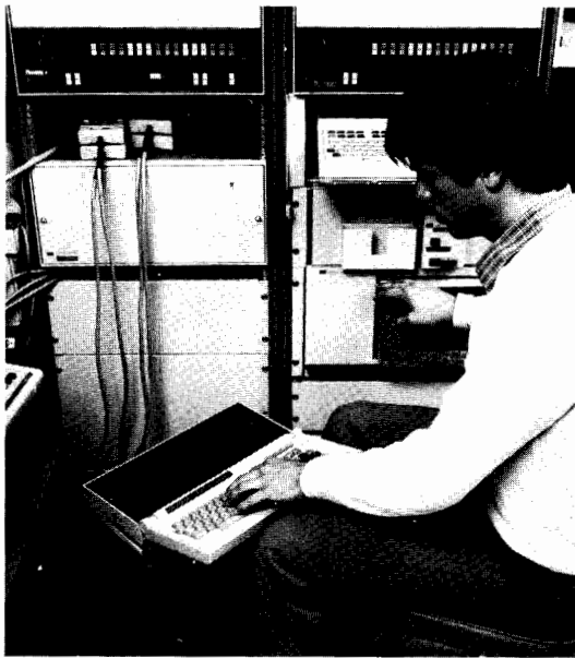
Figure 8. Model 64110A Development Station can be used at field sites and in product service for troubleshooting and service routines.
