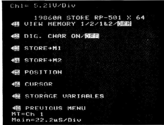
The intensified portion of the waveform is digitized with all 501 horizontal points.
