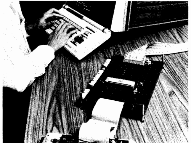
A user-definable emulator provides emulation support for microprocessors for which there are no processor-specific 64000 System emulators available.
