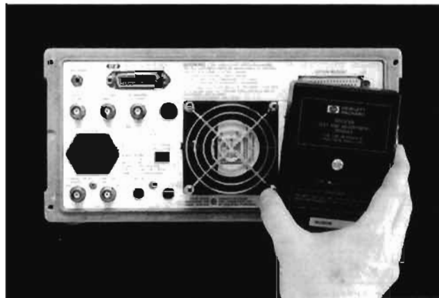
The HP 85629A Test and Adjustment Module plugs into the rear panel to provide extensive servicing capability.
