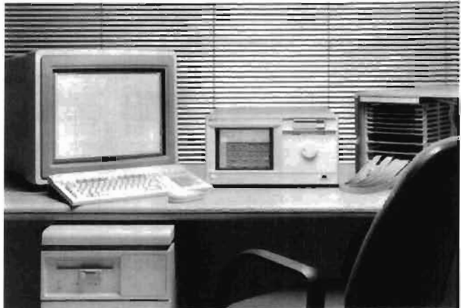
HP 74240A Electronic Design System-To-HP 16500A Logic Analysis System CAE Link.
