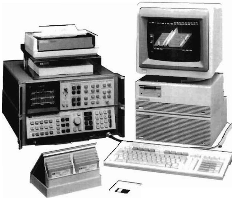
Typical system configuration using HP 85865B Signal Monitoring Software
