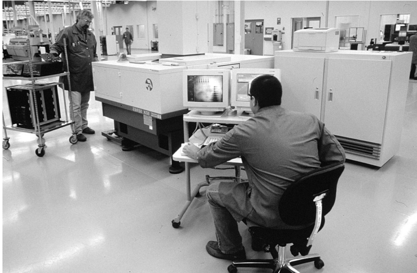
AXI locates process defects on densely-loaded boards with hidden joints.
