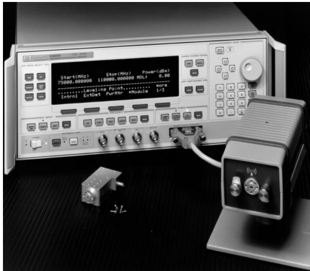
HP 83558A mm-wave source module. 75GHz to 110 GHz
