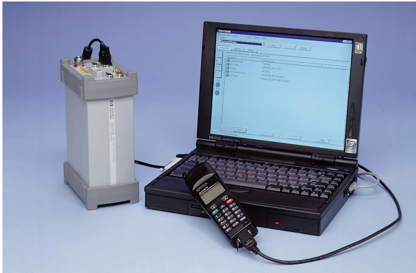
The new HP E74xx series provides measurements that optimize CDMA and GSM networks.
