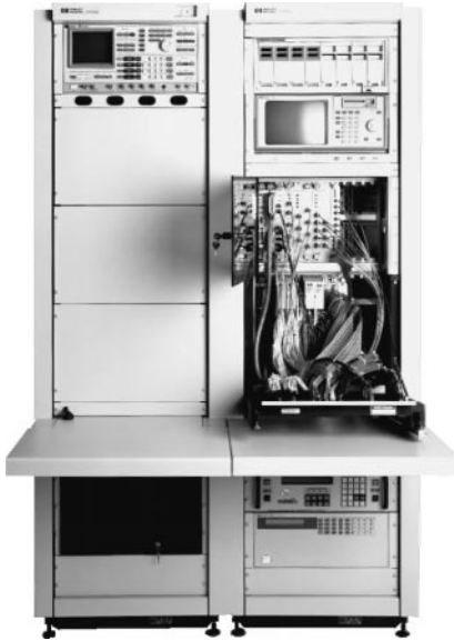
HP designed this VXI-based manufacturing test system with a high-density, quick-disconnect DUT fixture interface.
