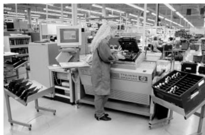
ICT finds an electrical class of faults, such as defective components and electrical circuit problems.
