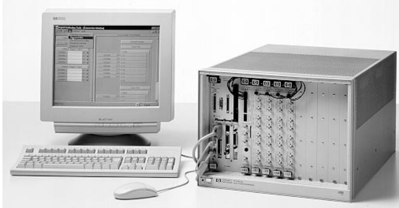
The HP 81200 Data Generator/Analyzer for characterizing complex multi-channel digital designs, shown here with the larger mainframe.
