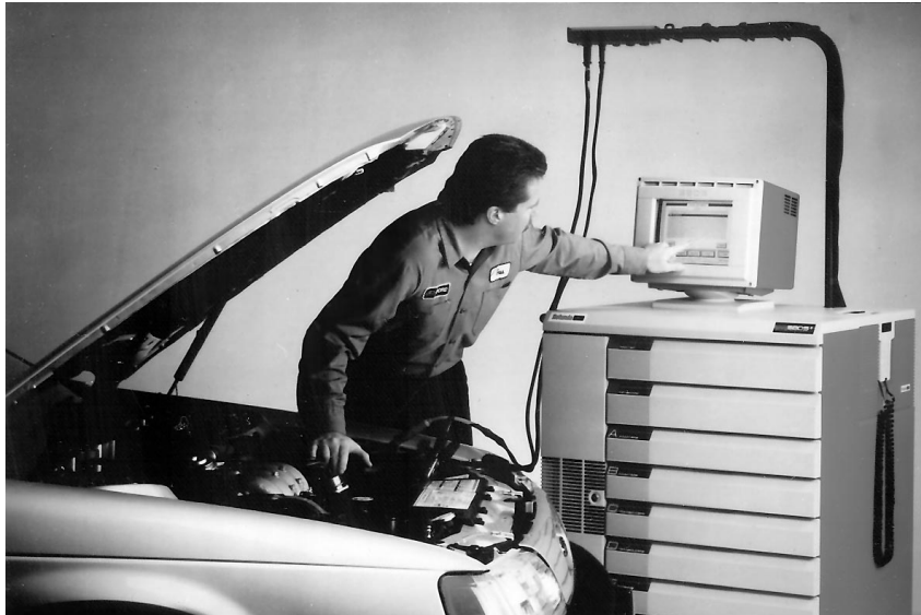
The Ford Service Bay Diagnostic System that HP helped develop combines computer-driven service tools and diagnostic strategies with on-line service information to save time and reduce repeat repairs.
