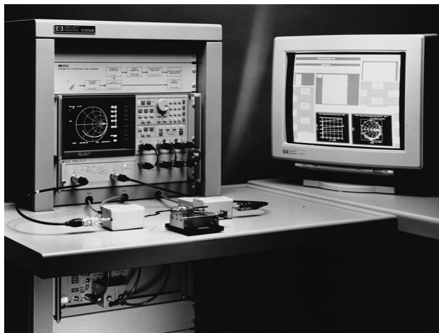
The HP 85123A RF Modeling System, together with the HP 85190A IC-CAP software, are shown extracting complete nonlinear models for RF active devices.
