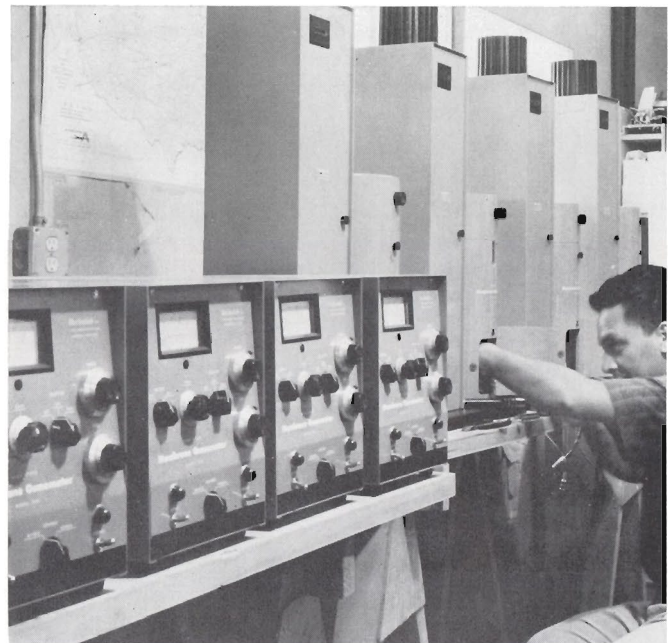
Assembly of four membrane high-speed osmometers nears completion. Instruments determine molecular weights of substances.
