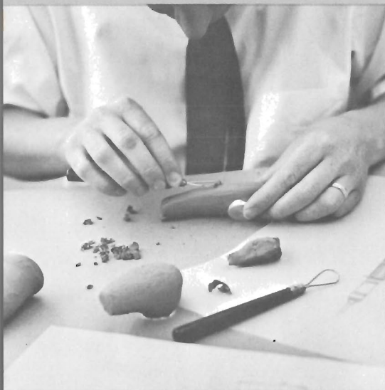
Component parts are sometimes mocked-up in clay before they reach final stage of design.
