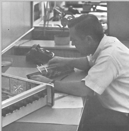
Here Rich Hoogner checks a cardboard mock-up of a proposed instrument readout panel.
