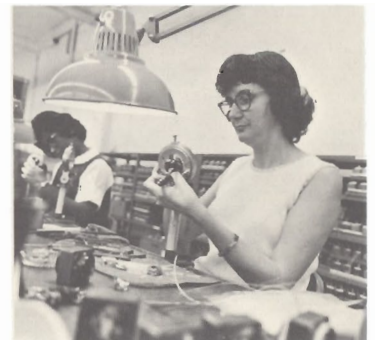
A coil for servo motor is wound by Dorothy Alexander.
