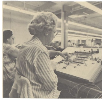
Mary Bottchen cables a harness with blueprint as guide.
