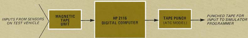
Figure 5. Technique for producing program tape containing simulated test course. Data obtained from an actual test course run are converted to digital punched tape representing all the parameters measured in the test run.
