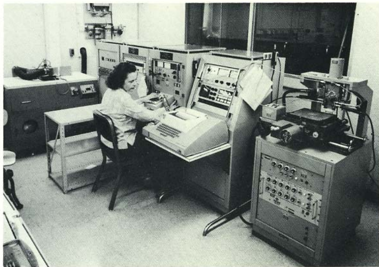
Figure 2. Thick-film circuits multi-testing facility is controlled by computer system behind window. Test stations, from left, are: functional abrader, special circuits, and automatic handler.
