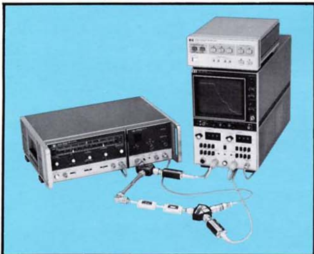
Figure 1. 105 dB Dynamic Range Measurement with the 8755.
