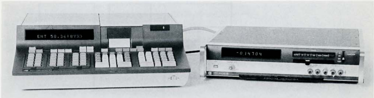
The 9820A Calculator is shown controlling a 3490A DVM using serial operation (the ASCII bus). The 3490A can be one of fifteen devices connected to the same bus. Each instrument on the bus is individually addressable.
