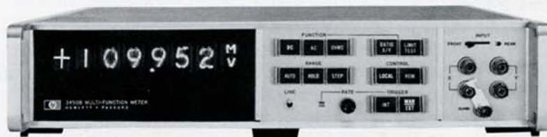
The hp-3450B is one of many Hewlett-Packard DVM's using the dual-slope integrating technique. The 3450B measures not only ac, dc, and ohms, but also has a four-terminal ratio input which may be used to measure the ratio of two independent, floating voltages.
