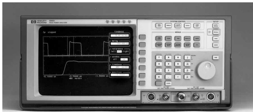
Figure 8-1. The HP 8990A peak power analyzer has two 500 MHz to 40 GHz microwave sensor channels and two video channels which provide for comprehensive characterization of RF/microwave pulsed power.
