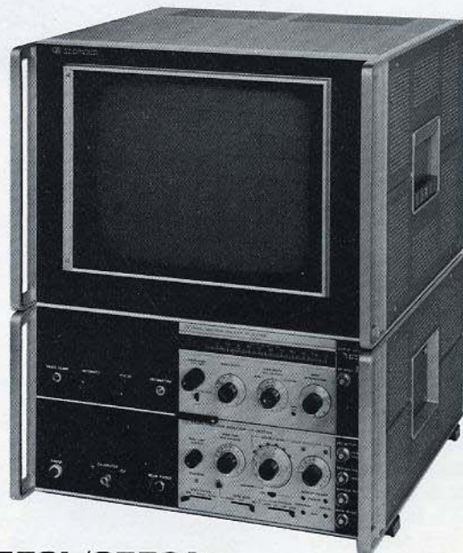
8553L/8552A with 143S Large Screen Display Section
