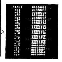
6. Press and hold in CURRENT MEASUREMENT DISPLAY section of the keyboard. The display moves up enabling you to view any part of the 64-state memory. When the end of memory is reached, an audible signal will sound, and a HARNING-CONDITION message alerts you that an operating limit has been reached; the display will roll no further. Release the ROLL DISPLAY key and the message will disappear.
