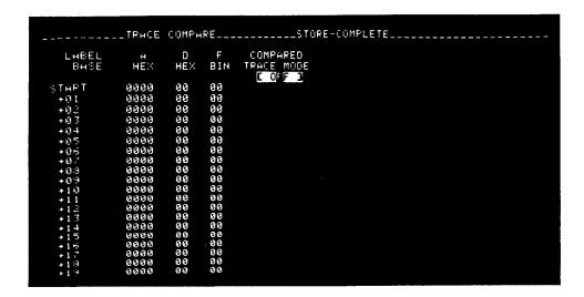
A separate rnemory in the 161 OA is provided for storing a known-standard data trace. This standard may be derived from the trace list by pressing the key in the EXECUTE portion of the keyboard. This key causes current measurement data to be stored in the "compare" memory,
