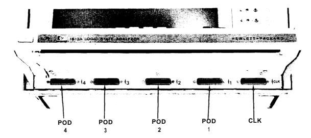
menu display **(see Chapter III)**. Each connector is keyed to the socket; the ridge in the molded plug should be on the left when being inserted in the socket. A spring clip on the connector locks it in position when it is pushed to the left as shown.
