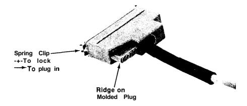
To insert plug into socket, slide spring clip to the right, insert plug in socket, slide spring clip to the left to lock in position,
