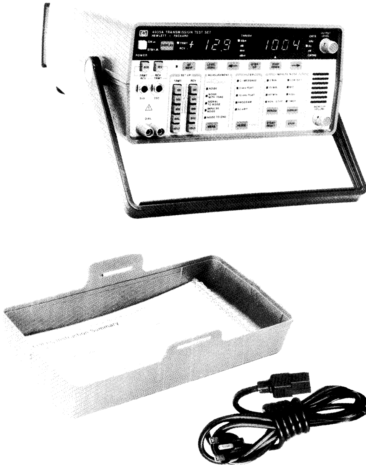
Figure 1-1. Model 4935A T ransmission Impairment Measuring Set
