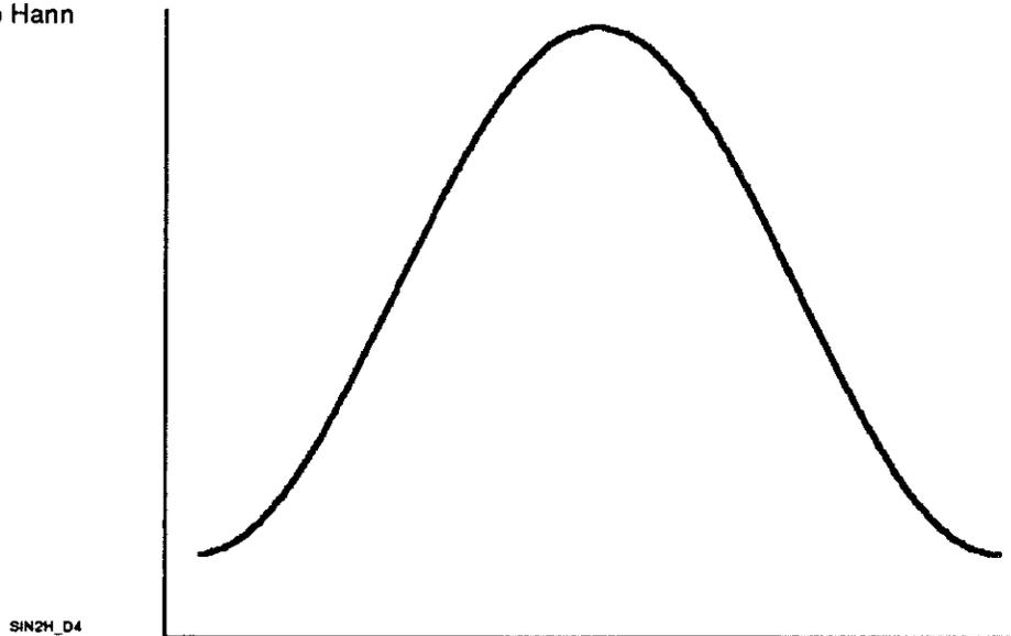
As you can see, the Hann window forces the endpoints of the sine wave to zero (which means they are equal). Although it appears to distort the original waveform, most of the amplitude information is still intact and the frequency information is virtually unchanged. The Hann window offers a good compromise between amplitude accuracy and frequency selectivity.
