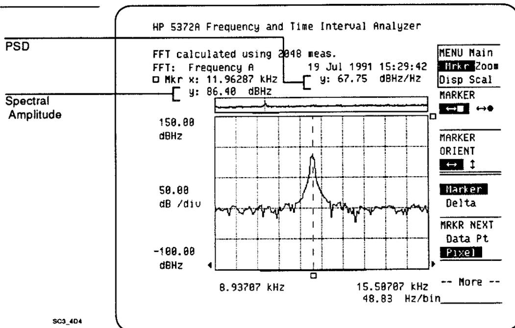
The PSD value is not provided directly over the HP-IB. To determine the PSD value over the bus, you would send the "PSDS?" query to return the power spectral density conversion factor. This value is to be subtracted from the original FFT results. In this example you would receive a value of 18.65. This value could then be used to convert the non-spur value to the PSD value. The same conversion factor applies to the entire FFT acquisition.
