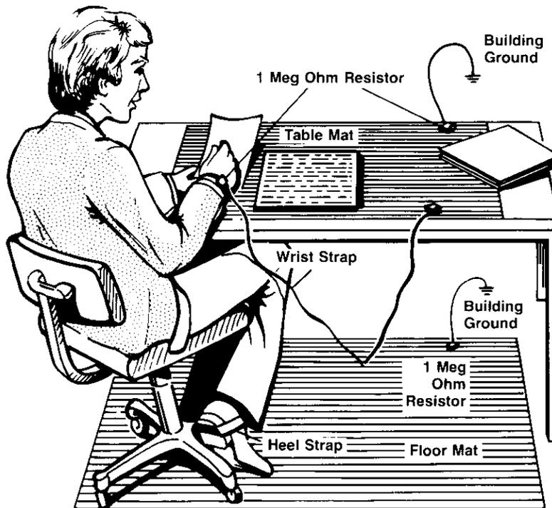
Figure 1. Example of a Static-Safe Work Station
