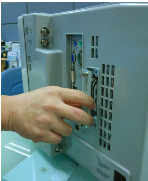
Figure 3-10 Pull and remove the hard drive from the slot
