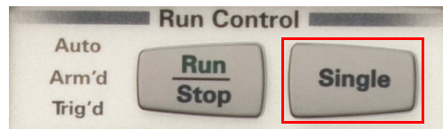
Figure 2-24 Single waveform acquisition button in the Run Control section
