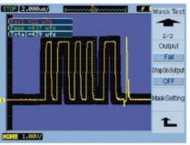
Mask testing provides a quick pass/fail comparison of an incoming signal to a test envelope you define.
