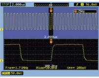
With True Zoom mode you can view a long record and the details of a zoom window simultaneously.
