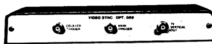
Figure 10b - three signal outputs on the back panel of the TV/video sync option provide access to the video signal, the main trigger signal and the delayed trigger signal. These signals are routed to a vertical channel, the main trigger input, and the delayed trigger input to view video signals.
