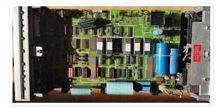
One of the EPROMs was loose and bouncing around inside the case. I first though that it may be that simple, but a closer look provided a much gloomier forecast. The EPROMs were infact in a small adapter boards, so someone has been here before. The adapter boards by themselves are not a problem, the Mostek ROMs in these units are known to fail and can quite easily be replaced by 2764 EPROMs, using an adapter to fix the pinout differences.
