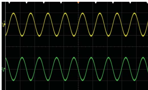
Figure 4. Tracked waveforms that are inverses of each other
