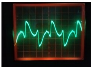
Waveform at the junction of V501 and V502 With red wire removed and 10mv applied to pin 13 of A6 board. 2ms/Div and 20mv/Div
