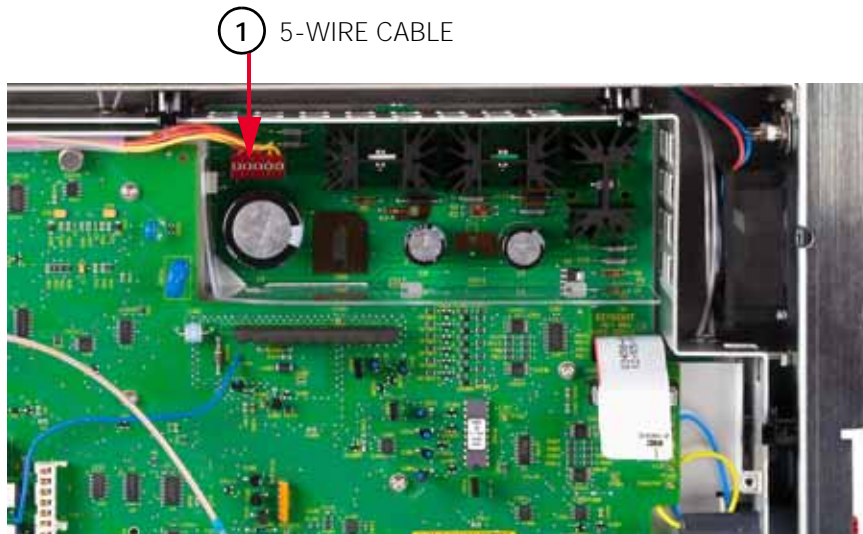
Figure 3-12 Remove/Install transformer cable on inguard power supply
