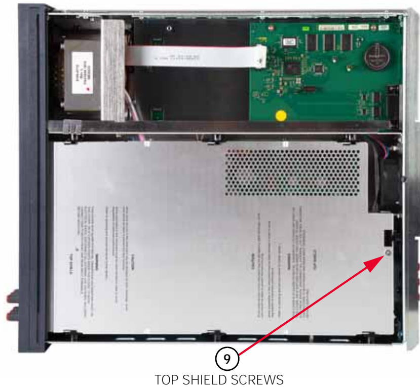
Figure 3-6 Remove/Install top shield screw
