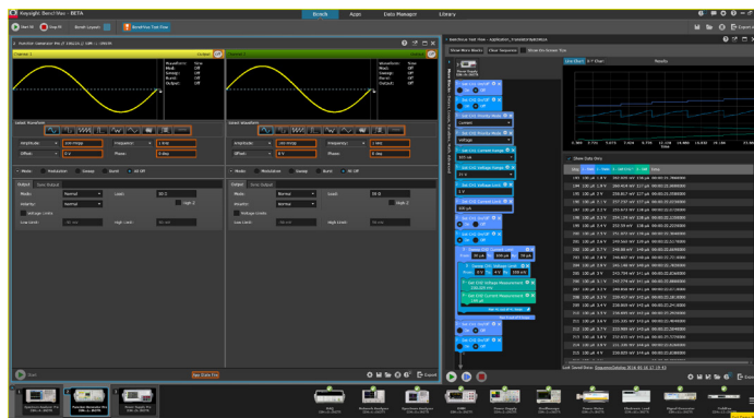
BenchVue Test Flow is integrated into the BenchVue framework and occupies the right-hand panel of the user interface.
