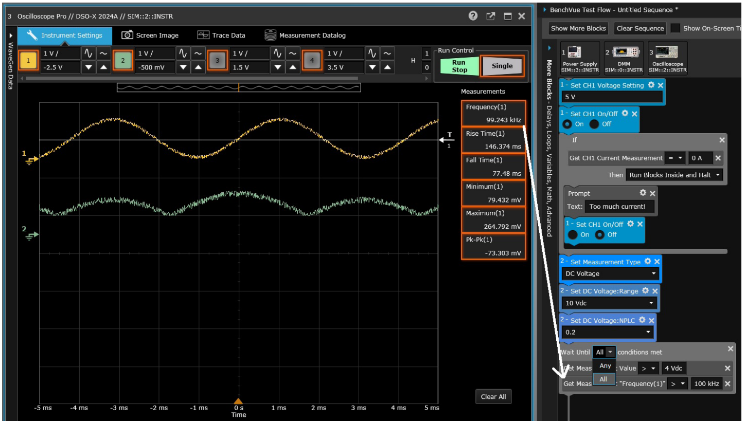
Figure 9. An oscilloscope measurement AND a DMM measurement are both used as conditions for testing to continue.
