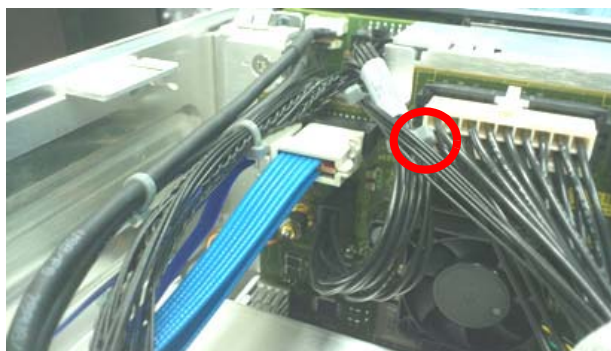
Figure 4-7 Measure potential relative to chassis at pin 9 of J12001
