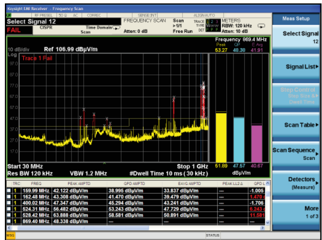
Figure 1-6. Radiated emissions plotted against CISPR11 limits as part of an EMI test
