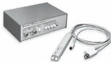
1141A 200-MHz differential probe with 1142A probe control and power module
