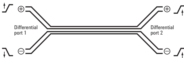
Figure 20: Mixed mode S parameters: S_{CD21} .
