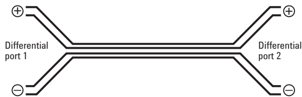
Figure 10. Differential line model.
