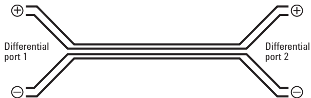
Figure 18: Differential S-parameter model.
