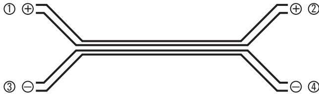
Figure 17: Single-ended S-parameters for a 2 port differential device.
