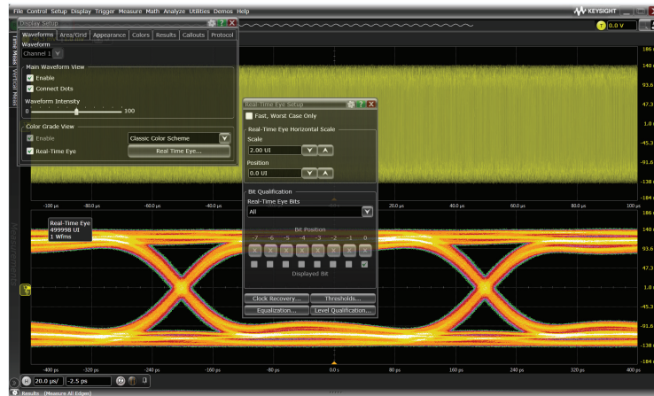
Figure 5. To set up a measurement, the wizard asks you to identify the signal source and select the clock recovery algorithm.
