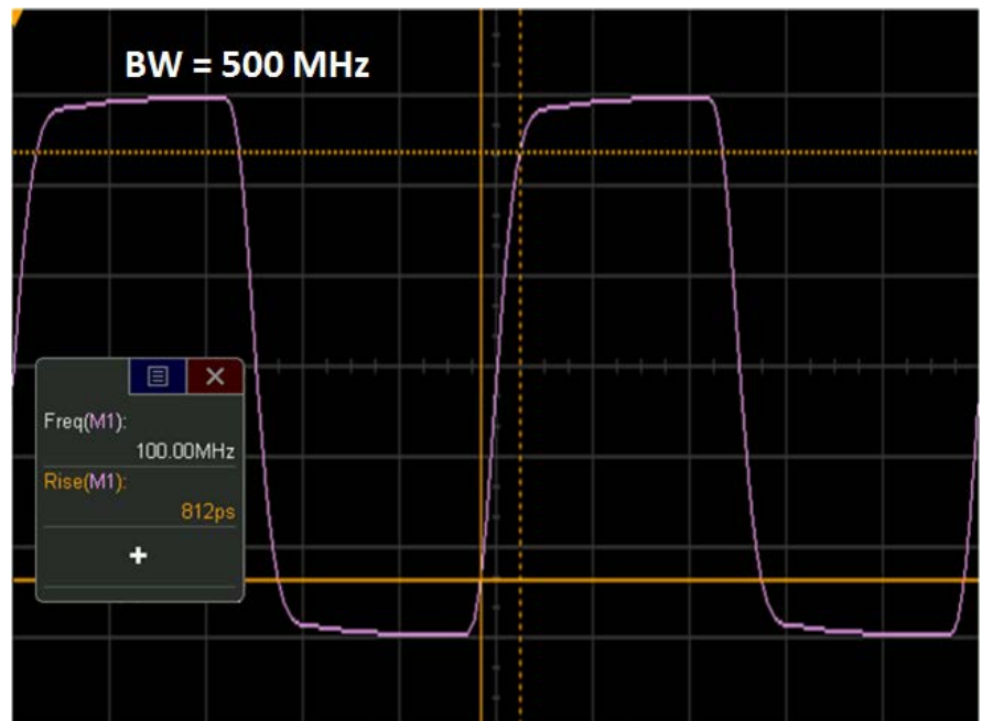
Figure 4: 100-MHz clock captured on a 500-MHz bandwidth scope
