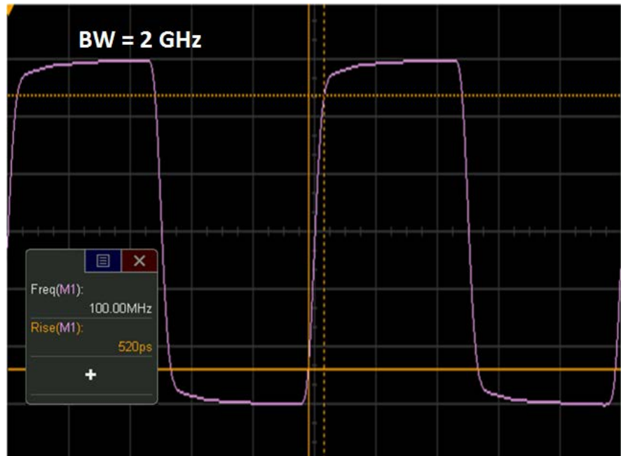
Figure 6: 100-MHz clock captured on a 2-GHz bandwidth scope
