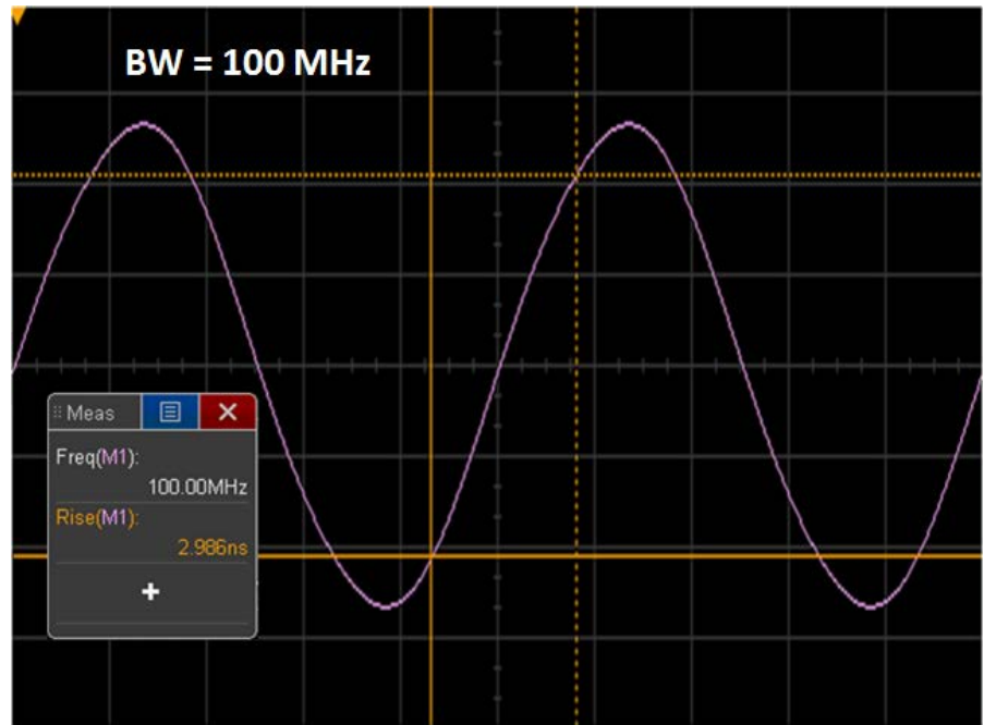
Figure 3: 100-MHz clock captured on a 100-MHz bandwidth scope
