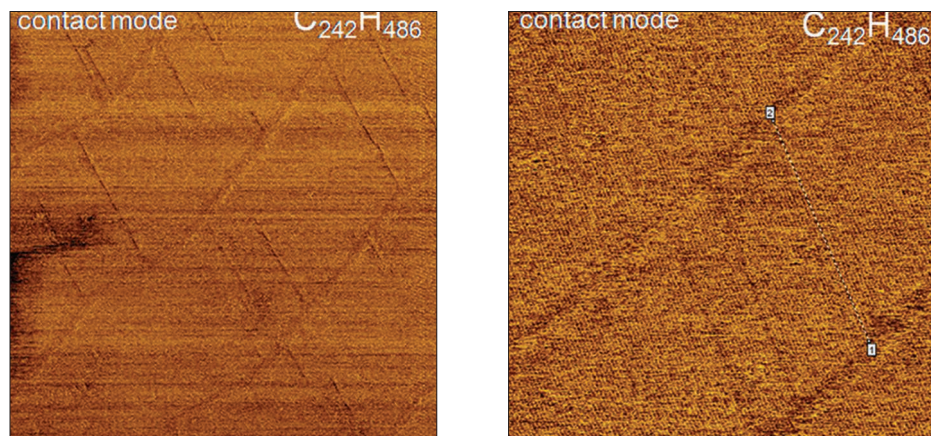
Figure 10. AFM images of C_{242}H_{486} lamellae on graphite obtained in the contact mode. Several slightly twisted lamellae were detected in the images of C_{242}H_{486} . A number of linear defects caused by the missing chains or their parts are also distinguished in the 100nm image (left). The individual alkane chains, which are extended between the edges of the lamellae, are also noticed in the 55nm image (right).
