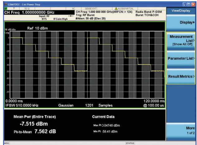
Figure 5. GSM list power step measurement for signal calibration using single acquisition combined measurement mode.
