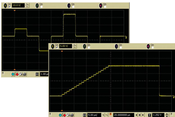
The arbitrary linear waveform generation capability of the 4082F's HV-SPGUs makes it easy to create complex waveforms.
