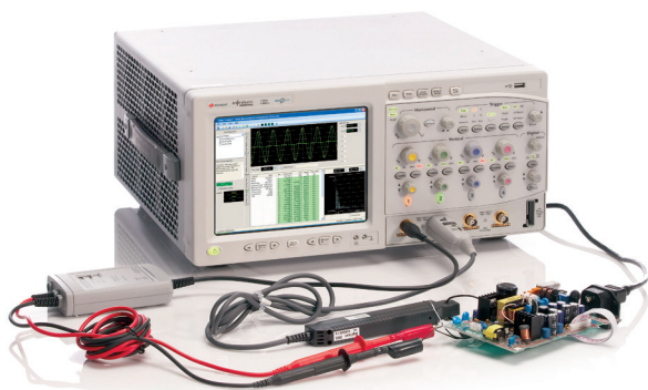
Figure 1. Power measurement application running on a Keysight 8000 Series oscilloscope provides a single-box solution for testing switching mode power supply characteristics
