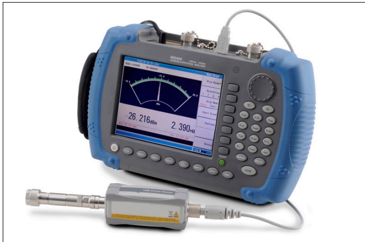
Figure 13. HHSA connect with USB power sensor.
