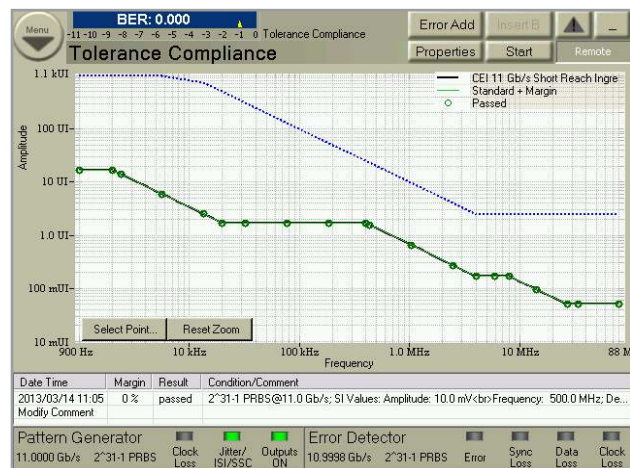
Figure 5. Result screen of the automated jitter tolerance compliance. A library of jitter tolerance curves is available
