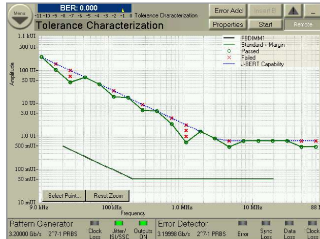
Figure 4. Automated jitter tolerance characterization. The green circles show where DUT works within the required BER-level
