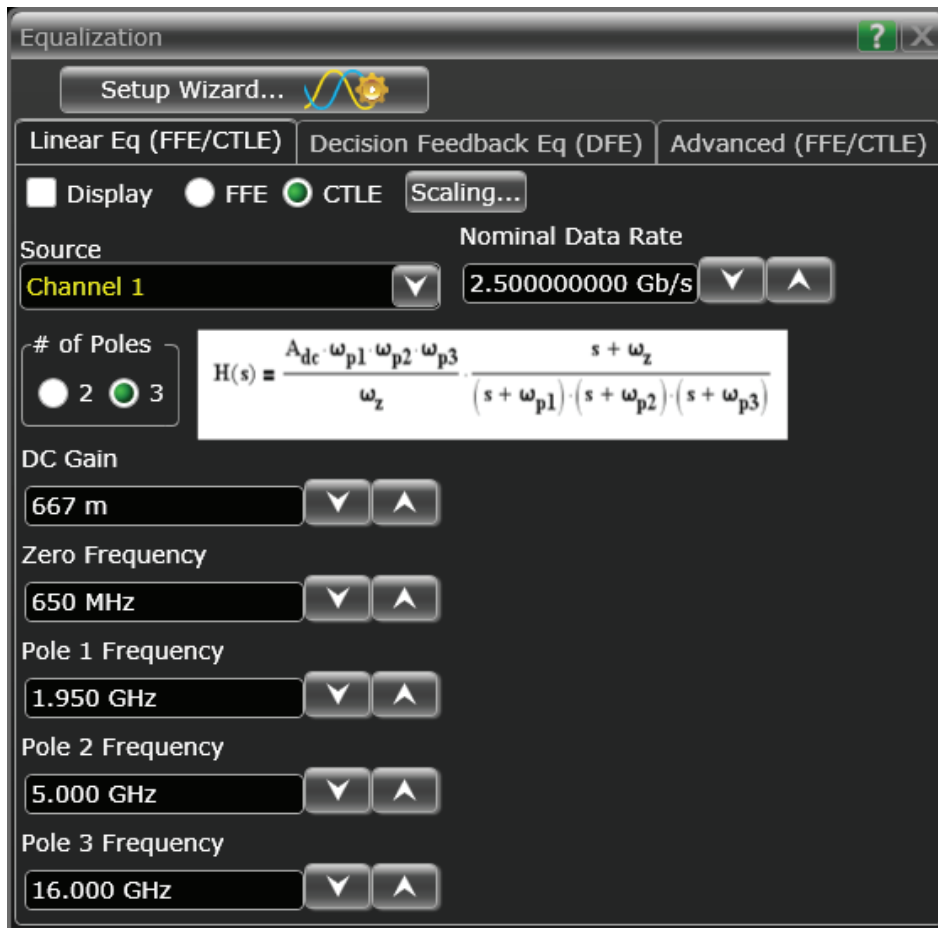
Figure 6. Serial data equalization supports both 2- and 3-pole CTLE
