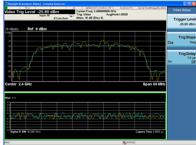
Figure 16. IQ analyzer display with 40 MHz analysis bandwidth
