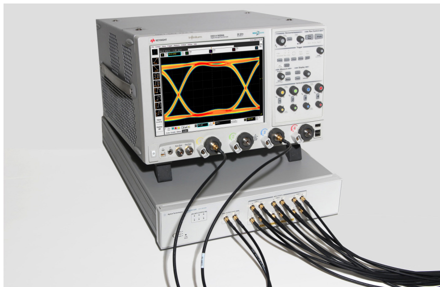
Figure 17. Automated testing for multi-lane digital bus interface through switching solution
