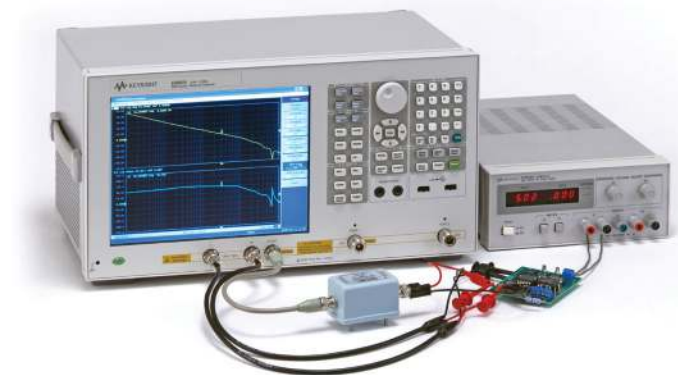
DC-DC converter loop-gain measurement with gain-phase test port
