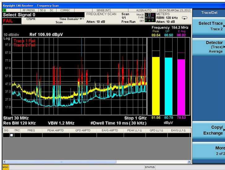
Figure 9. Swept traces in both clear write and max hold trace types; whip antenna length was changed during the sweep to simulate antenna height scan, resulting in the difference between the traces
