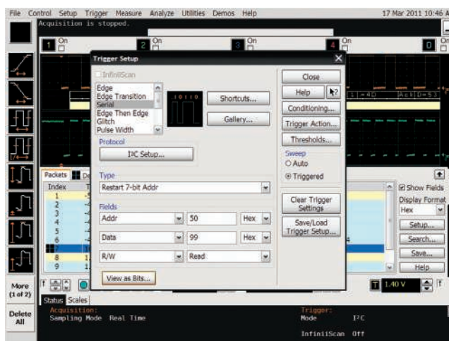
Figure 9. I 2 C trigger setup on a 9000 Infiniium Series oscilloscope
