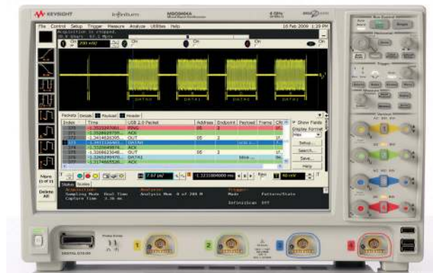
Figure 1. Three instruments in one – a 9000 Series oscilloscope with built-in protocol analysis for USB, I 2 C, RS-232, SPI, CAN, FlexRay, and PCI Express
