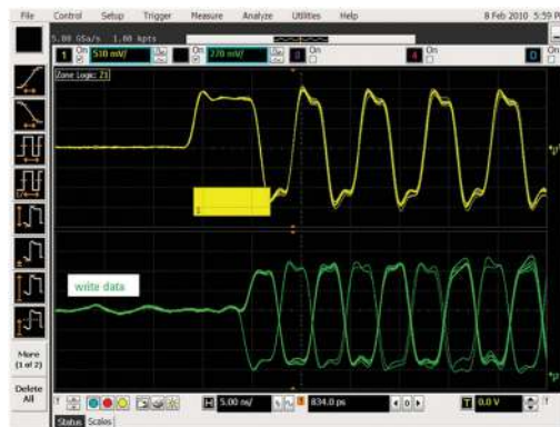
Figure 4. Using InfiniiScan software's zone qualify trigger enables you to trigger on read or write bursts to separate read and write data for eye diagram testing. Read data is edge aligned with the strobe while the write data is center aligned with the strobe.
