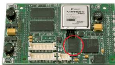
Figure 3. Limited space in embedded boards and computer systems means more DRAMs are packed into a DIMM configuration to enable higher capacity.
