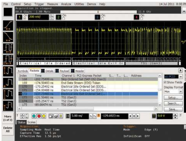
Figure 3. The packet-level decode below the correlated portion of the PCI Express signal
