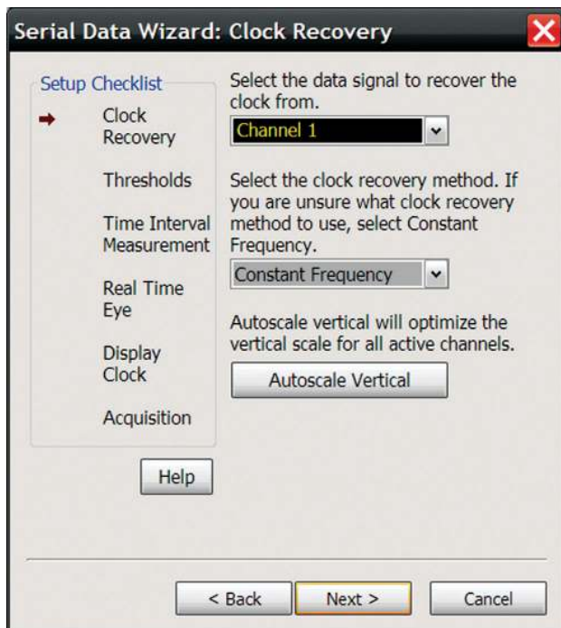
Figure 1. To set up the decode, the wizard asks you to identify the signal source and select the clock recovery algorithm (constant frequency shown. 1st and 2nd order PLLs can also be selected).
